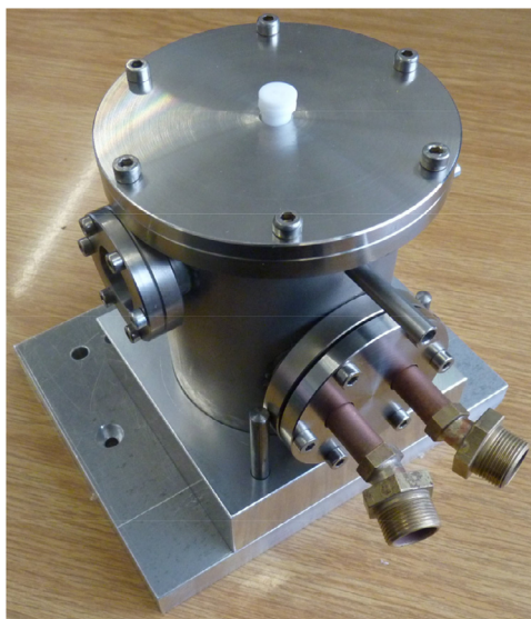
Fig. 7. Housing of the measurement chamber with closed lid and liquid cooling connectors. The sample can be manipulated without breaking the vacuum.
